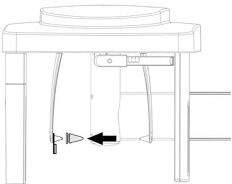
7. Secure the contrast element using a hygienic cap.
