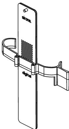
8. Attach the ceph test phantom to the clip provided for that purpose.
