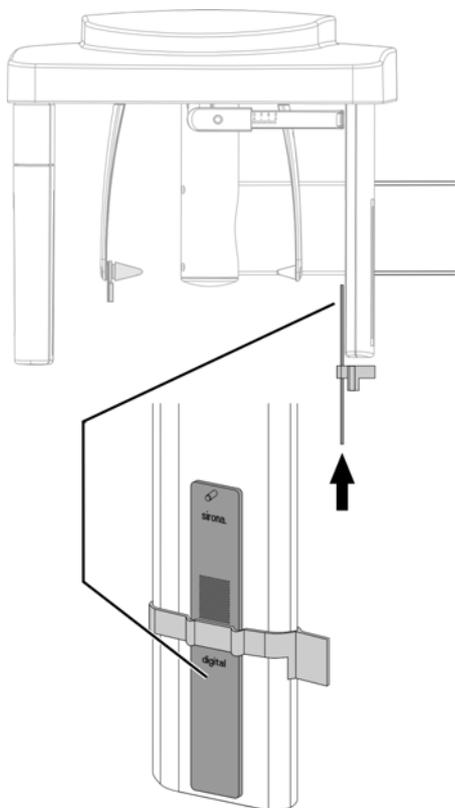
9. Push the ceph test phantom with the clip from **below** on to the secondary diaphragm of the ceph arm.
