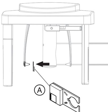
6. Fit the contrast element **(A)** with its hole onto the ear plug.
