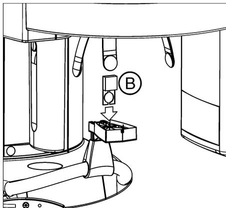
2. Plug the contrast element (B) into the slot on the needle phantom provided for that purpose.
