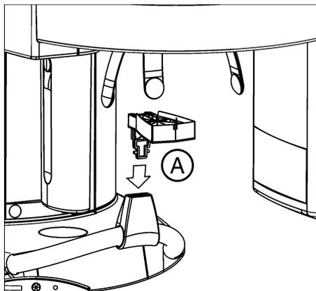
✓ The panoramic sensor must be plugged into the sensor holder.
