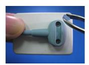
Using tweezers, remove a gel disk from its paper backing and place it over one of the screws you just tightened. Make sure that the gel material completely covers the screw. Remove another gel disk and repeat this action for the second screw.
